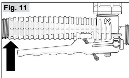
To spray, depress the hand lever on the valve.
