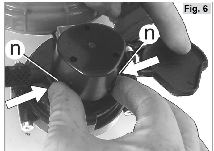
To remove the rechargeable battery from the device, compress the two latching levers (n) to unlatch the battery, and then take out the battery upwards.
